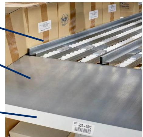
IL SISTEMA DI PICKING DINAMICO PUÒ ESSERE CONFIGURATO IN DUE MODI, COME INSTALLAZIONE COMPLETA O COME PARTE DI UN IMPIANTO PORTAPALLET O SCAFFALATURA PICKING MANUALE, POSIZIONANDOSI AI LIVELLI INFERIORI.
